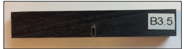
Fig.7. Example of SENB sample ready for test.
