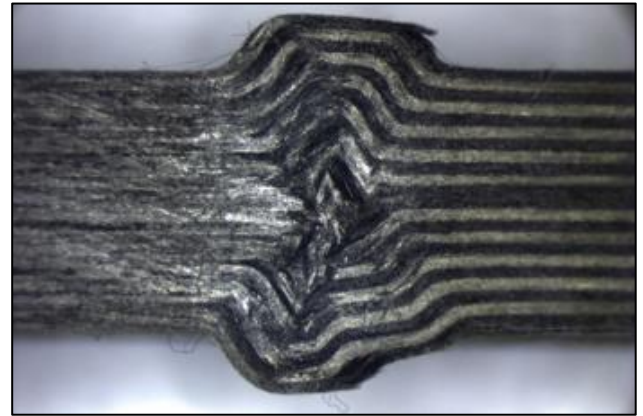
Fig.16. Top view of samples with a fibre orientation \pm 80^\circ to crack plane after testing.
