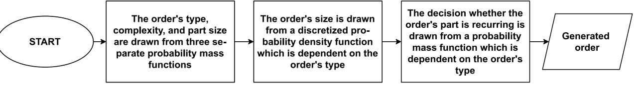
The process parameters are directly affected by the currently processed order's composition. E.g., if the order's complexity level is high, then CAM, tool preparation, setup, and CNC milling is likely to require more time than orders of lower complexity. The method for generating the process parameters can be seen below:
