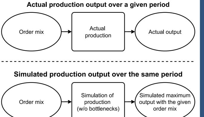
Thus, if the simulation reflects the production without bottlenecks, it can simulate the maximum output for the given order mix. Once the actual output and simulated output has been achieved, these numbers can be used to compute the theoretical performance of the current system. An array of input parameters and process parameters are required to setup a DES with sufficient quality and accuracy. These parameters have been identified as the following:
