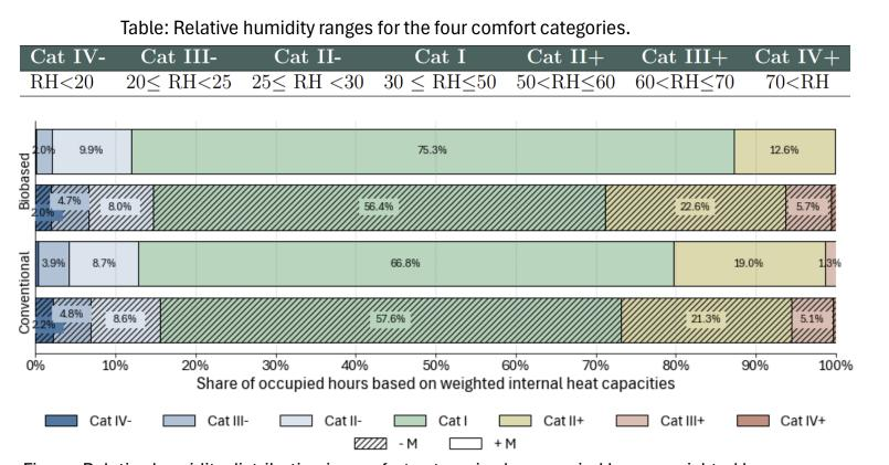
Figure: Relative humidity distribution in comfort categories by occupied hours, weighted by internal heat capacity, for one room type in conventional and biobased constructions, when moisture dynamics are excluded (-M) or included (+M).
