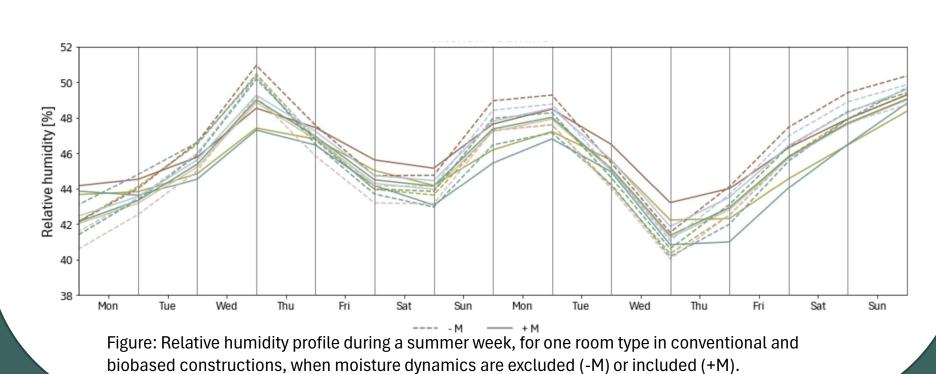
• Biobased materials have a higher moisture capacity, but is does not compensate for their reduced heat capacity. They can only match the thermal performance of heavy conventional constructions to a limited extent. This limitation applies if indoor temperature is not to be effected.
