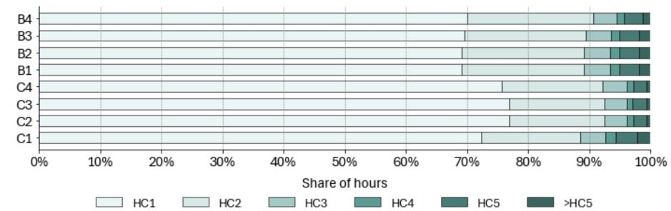
Figure: Share of hours in the different humidity classes, for one room type in conventional and biobased constructions.
