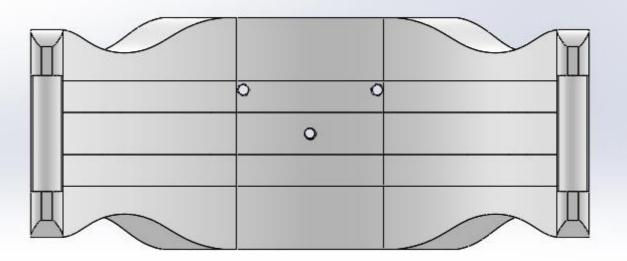
With this final geometry, two simulations are carried out. The first one is with the Ansys ACP tool to analyze the composite material, and according to the Tsai-Wu criterion, the structure does not fail for the given static load case. As for the simulation with PLA, a maximum stress in the central hole area of 10.874 MPa is obtained, which is less than the yield strength limit of the material, being 70 MPa, i.e. it would not fail for the same load case.
