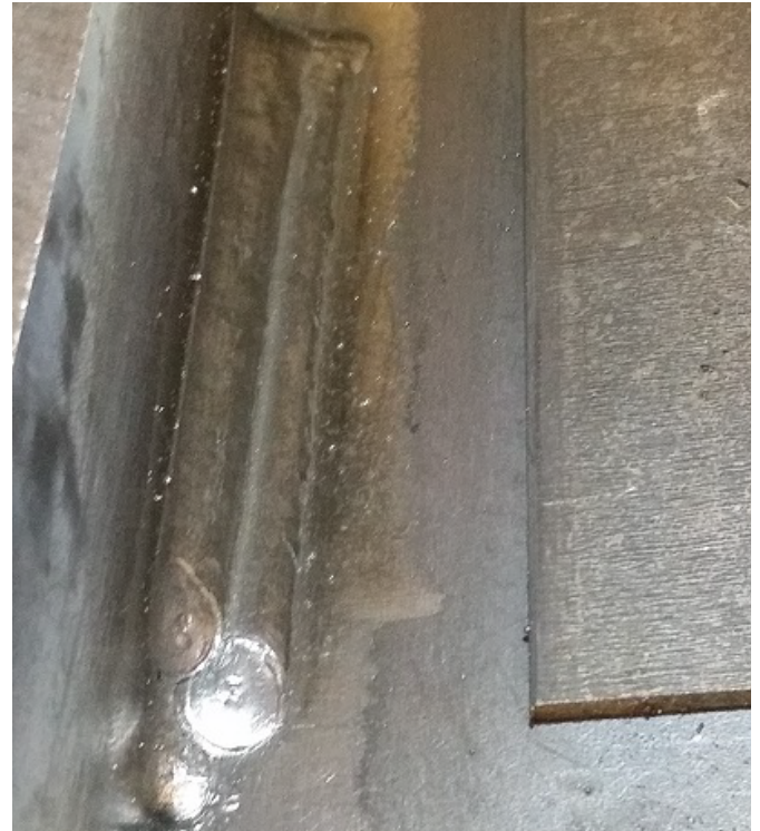
Fig. 5 Macroscopic image of a multiple pass weld sample. This initial visual inspection of the weld determines, if large surface defects are present in the weld.
