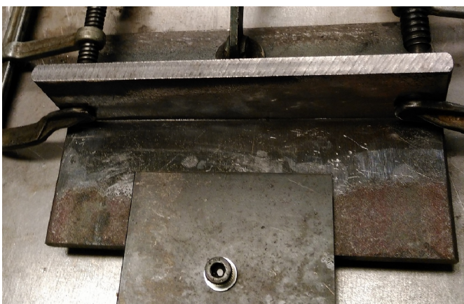
Fig. 3 Simple fixture for fixation of the parts.
