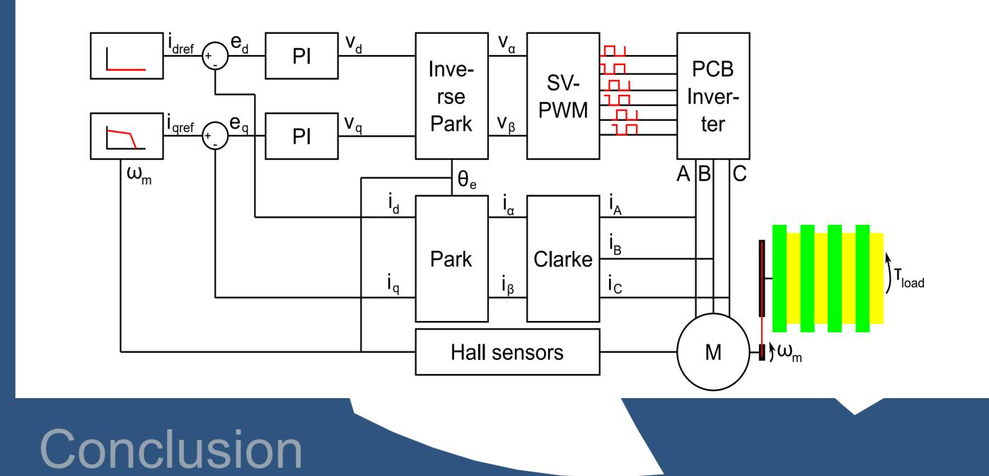
It can be concluded that the project has done a redesign of the drive train for the Cowbrush unit. The redesign implements a new belt trans mission with a PMSM, where a DSP and corresponding PCB utilizes a
