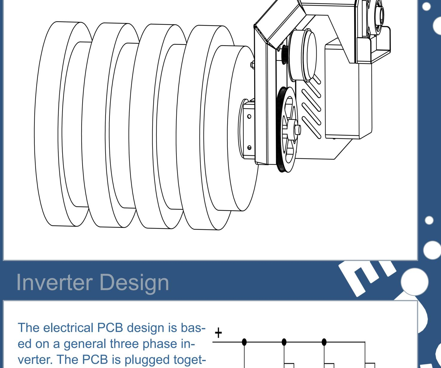
A Field Orientated Control structure is established for the system, which drives the system with a desired torque control. The torque is controlled by two PI controllers that regulates the currents, that transfer into a smooth operation of the brush seen from a cow.
