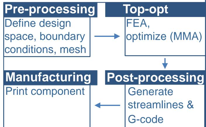
**Path-planning** via streamlines generates manufacturingtolerant paths, that follow optimized orientations. Gaps and discontinuities are present and should be minimized by novel techniques. From the **streamline method**, a specimen of the **optimized**
