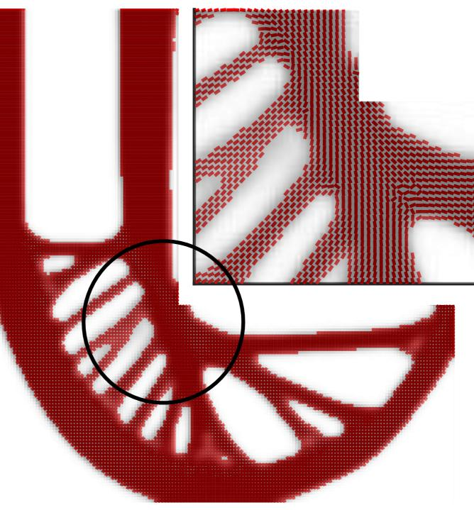
The fiber angle filtering smooths fiber orientations, resulting in increased manufacturability. The principal stress directions and fiber orientations are primarily aligned.
