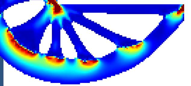
**Mass-constrained optimization** minimizes the compliance. However, it results in a stress concentration, where failure is predicted.
