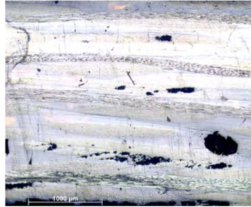
**Fig. 20** Microscopic image of the section perpendicular to the resin flow of the composite spar.
