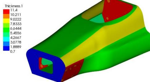
Thickness is not always proportional to weight. Results from ANSYS simulations showed that sandwich structures give higher stiffness to the monocoque. A less dense and thicker core material (PVC) was used to reinforce the weaker parts.
