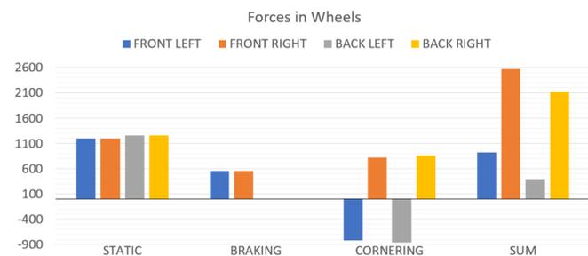
To analyse the torsional stiffness of the monocoque the maximal force from front left wheel  $F_{yrr}$  multiplied by a dynamic scaling factor of 3 have been used.
