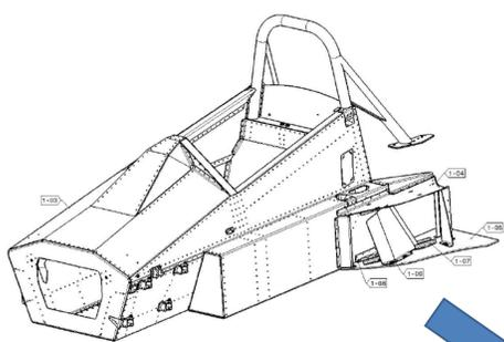
The redesign resulted in a more smooth geometry offering good stress distribution around the cockpit without using front roll bar.
