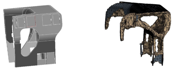
Fig. 9 Result from topological optimization for torsion.
