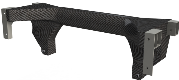
Fig. 15 Design of the new rear subframe for the Agile SCX.
