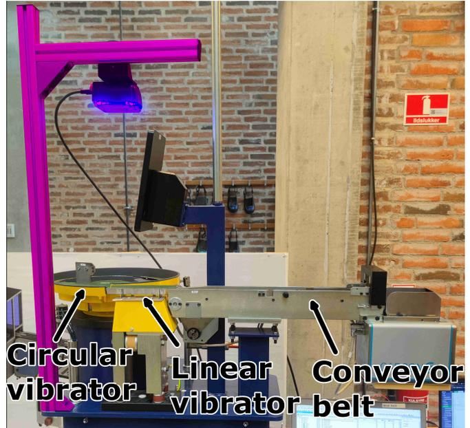
Fig. 4 The camera installed on the vibrator (mount with camera marked as magenta)
