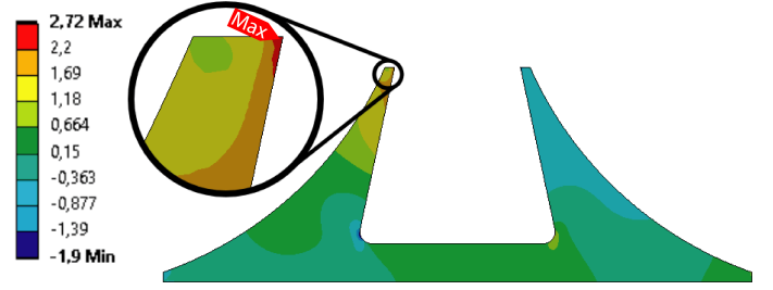
Fig. 6 Shear stress-field in MPa in the connection piece.
