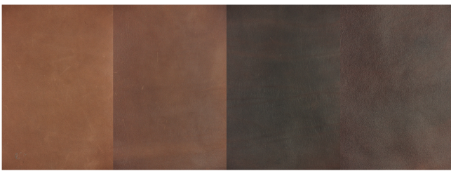
Fig. 6 A closer comparison of the samples. Untreated, brushed, creamed and polished.
