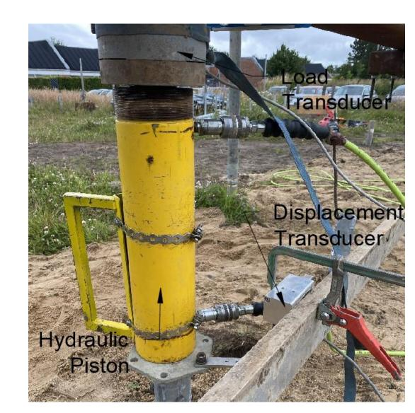
The force applied at 40 mm data from static load test is used in a semi-logarithmic linear correlation to describe the relationship between time and bearing capacity. This analysis is applied to piles with varying geometric parameters. Statistical evaluation is performed on compression test data at a depth of 7.8 meters, and the mean values of the confidence interval are presented in the figure below
