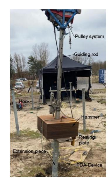
The dynamic capacity is generally evaluated through an energy consideration. In Denmark, it is most common to use The Danish Driving formula (DDR) for evaluating the dynamic capacity. The dynamic capacity have been evaluated using measured results from dynamic load test, along with DDR. A relation between the static capacity and the dynamic capacity has been found, and a comparison between evaluated static capacities and measured static capacities has been computed as illustrated below.
