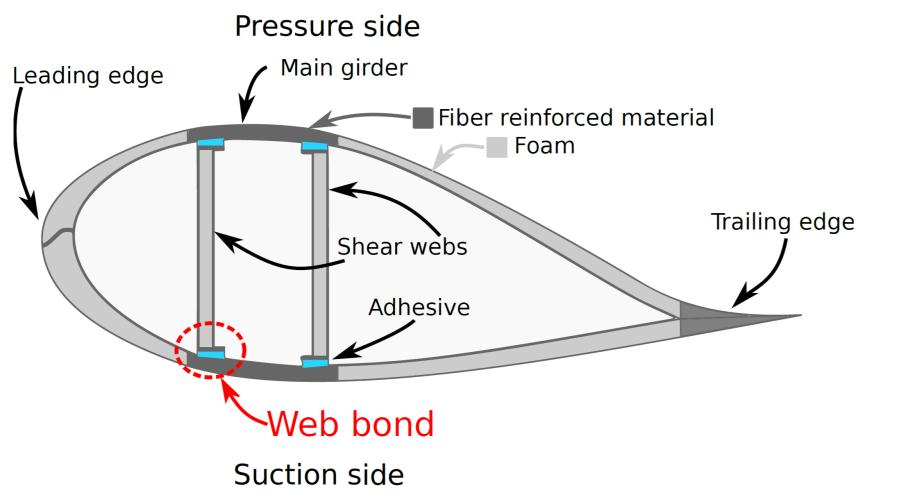
Following the latest design guidelines for the wind blade industry [2], the load capacity of an initial design of the web bond detail is investigated through testing and modeling. It is then optimized and validated through further testing.
