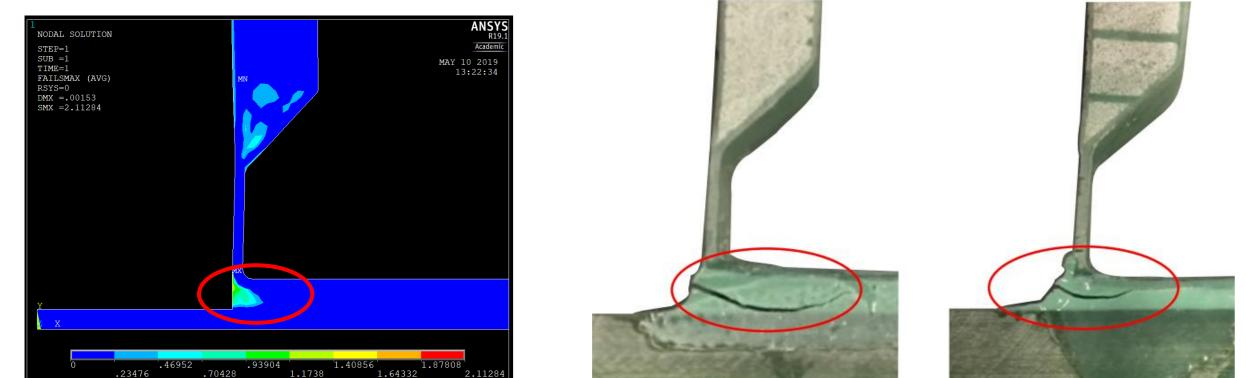
The results of the testing were compared to a tailored structural analysis of a submodel replicating the different experimental load cases. Failure indices based on the max stress criterion were extracted from the FEM analysis, thus providing the failure envelope of the initial design of the web bond detail.
