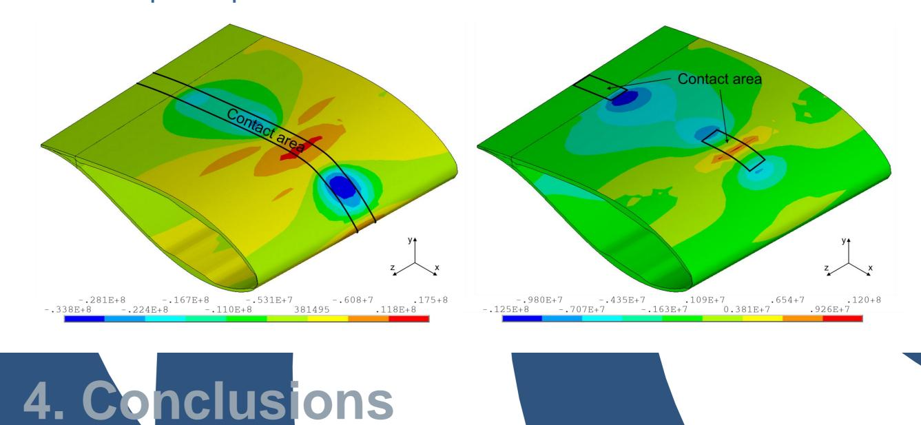
In this study it was found that five yokes should be used when a full scale test of this blade is done. It was further found that applying the loads through the yokes only had a minor global stiffening effect on the blade. Regarding the local effects, it was found that the invalid region comprising 75% of the chord length in the spanwise direction can be reduced. However, an exact value cannot be defined due to modelling limitations, and further studies must be done.
