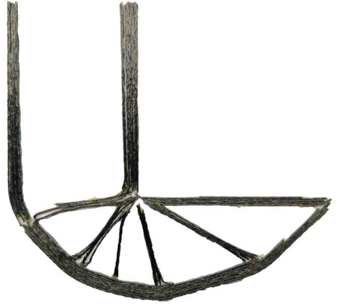
Fig. 9 The 3D printed CFRP specimen based on the topology optimized design in Fig. 7.
