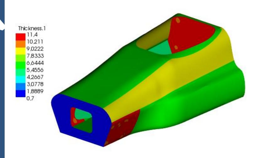
Thickness is not always proportional to weight. Results from ANSYS simulations showed that sandwich structures give higher stiffness to the monocoque. A less dense and thicker core material (PVC) was used to reinforce the weaker parts.
