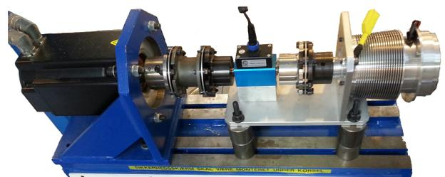
Fig. 21 Load motor (left), torque transducer (center) and PMSM (right).
